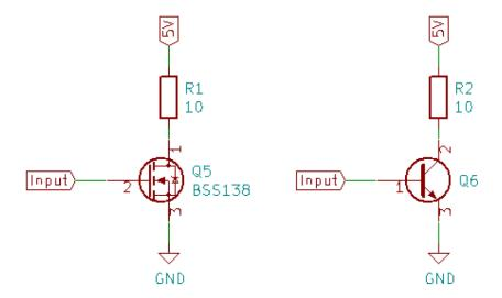
(c) Now you control the FETs with an Arduino microcontroller connected to the input. An Arduino can produce voltages between 0 V and 5 V. Can you switch the light on/off?
