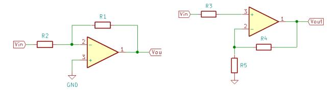
(b) Here is an op-amp symbol with the supply voltages visible. Let's consider again the circuits above, but with  $V_{S+} = 5 V$  and  $V_{S-} = 0 V$ . In case of an ideal op-amp, what would the output voltages limits be? What about for a real op-amp?
