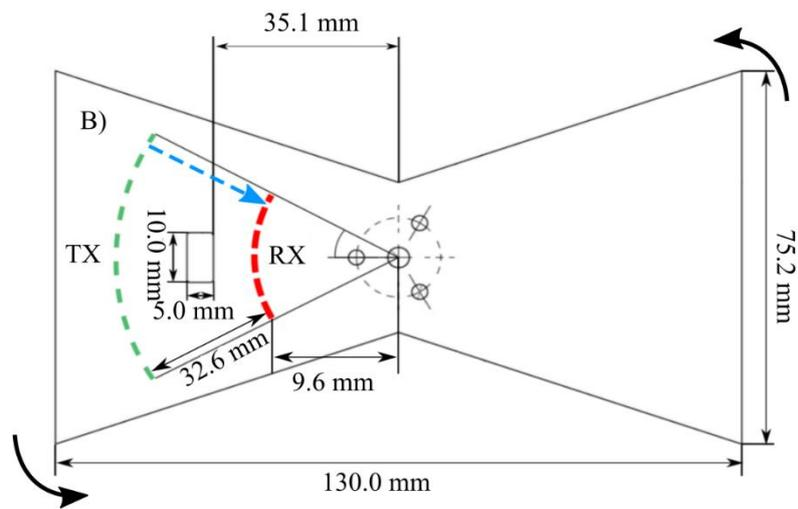
Assume that the propeller is  $130 \times 75.2 \times 4 \text{ mm}^3$  in size, the group velocity of the fundamental antisymmetric mode in the undamaged region  $v_g = 3180 \text{ ms}^{-1}$  and in the damaged sector  $1686 \text{ ms}^{-1}$ . Following the figure calculate the time difference on the arrival of the Lamb waves (blue arrow) between the waves that travel in the intact region to those that propagate through the defect.
